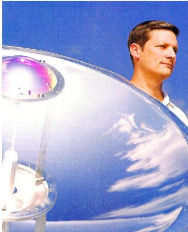
Duncan Earl (Sunlight Direct) says his new system is far more efficient than lights drawing solar power from photovoltaic cells. These convert photons to electricity and electricity back to photons, wasting 98% of the sunlight's original energy.
